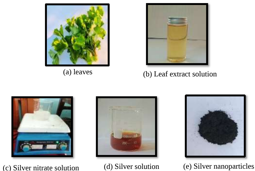
Figure 1. Synthesis procedure of green synthesis of silver nanoparticles
